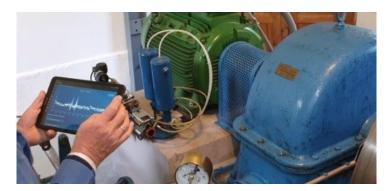
In addition to expert visual observation, intelligent plant tuning also includes analysis and evaluation of the data from the machine control system. The result is a comprehensive view of the actual condition of the machine or system and thus an optimal basis for planning targeted maintenance operations. Thanks to automated machine data recording, deviations from the normal state are detected at an early stage by means of trend analyses.
