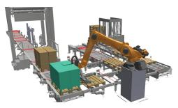
Retrofits can bring machines up to the latest state of the art. With a continuous simulation, it can be evaluated before the retrofit which improvement can be achieved by a retrofit.
