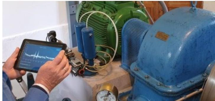
In addition to expert visual observation, intelligent **plant tuning** also includes analysis and evaluation of the data from the machine control system. The result is a comprehensive view of the actual condition of the machine or system and thus an optimal basis for planning targeted maintenance operations. Thanks to automated machine data recording, deviations from the normal state are detected at an early stage by means of trend analyses.
